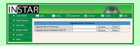
While updating the firmware, you should never disconnect the power from the camera because it will cause serious damage to the camera. In the worst case you will not be able anymore to use the camera. The update of the firmware should only be done after contacting your distributor/dealer.
