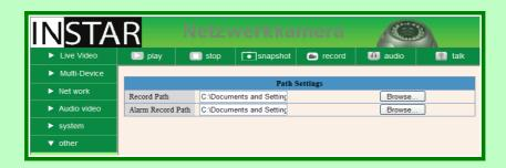
The "Record Path" will be used for the manual recording in the web interface.
