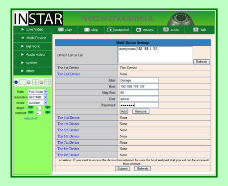
The first camera is always the camera which you are currently configuring. All cameras which can be found in your network will be shown in the box "Device List in LAN". You can add a camera if you enter the following settings:
