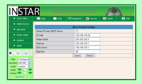
The option "Obtain IP from DHCP Server" will cause your camera to receive its IP address, Subnet mask, Gateway and DNS Server information from a DHCP Server in your network. This is mostly done by the router in your network. We recommend you to not use this function since the camera might get a different IP address over the time so that it will not be possible anymore to enter it via Internet without also changing the routers configuration. Therefor it is better to set the IP address manually.
