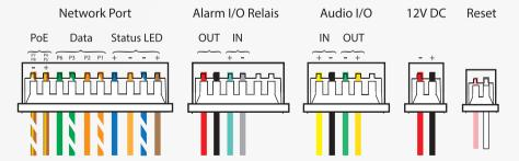
The installation of the new cable is very simple. The cable order is identical to the original one and is already placed in the right order. The plugs have different connector sizes and will only fit into the earlier unplugged connectors.
