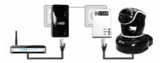
It is not recommended to plug the device into a power strip with surge protection or into a UPS. Both sockets have to be a part of a single circuit - make sure that there are no circuit breaker or electricity meter in between.
