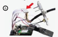
Now plug the heater element to the now vacant connector on the mainboard (Fig. 5). Then connect the other end of the cable from the heating element with the 13-pin power supply (Fig. 6). Please make sure that all plugs are properly connected. To reassemble the camera you will need to reattach the mainboard to the back cover (Fig. 3) and reconnect the mainboard with the sensor unit. (Fig. 2).
